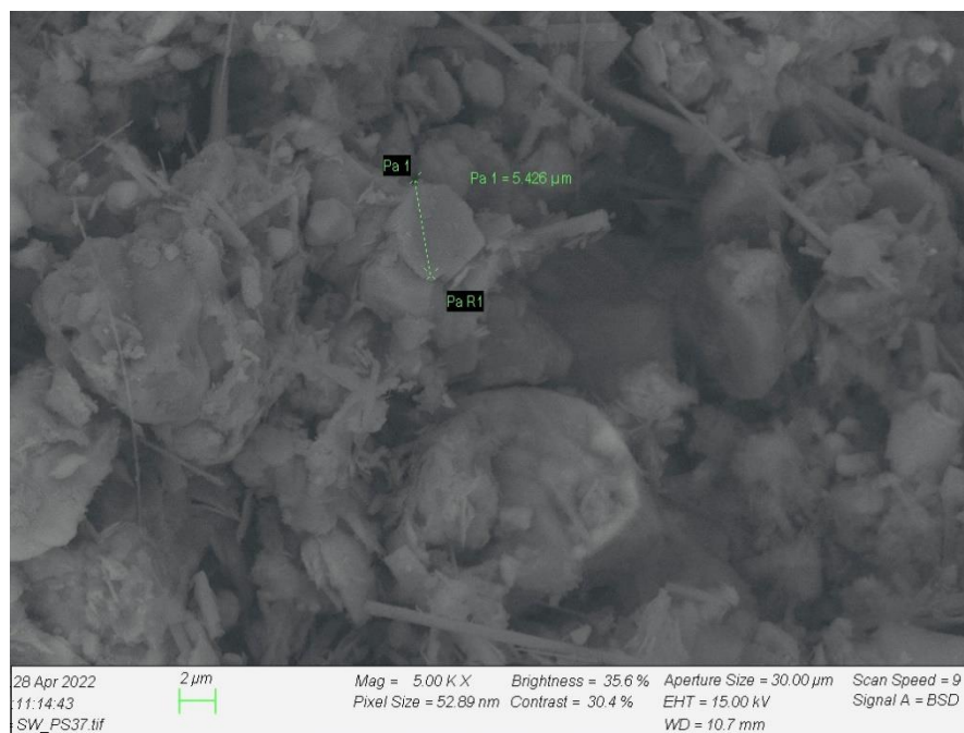
Figure 39: SEM image of the salt residue from SW-PS at 5000 x magnification
