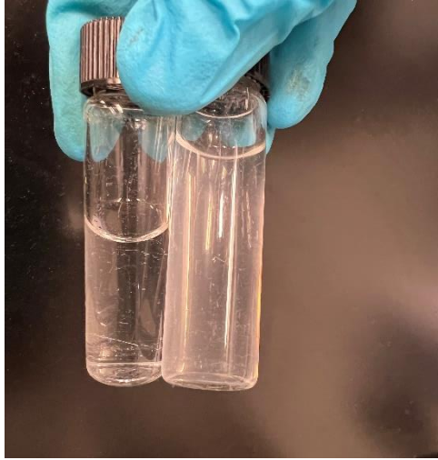
Figure 30: Batch test showing a blank sample (left) with no precipitation of BaSO_4 and a cloudy sample (right) indicating precipitation of BaSO_4 .
