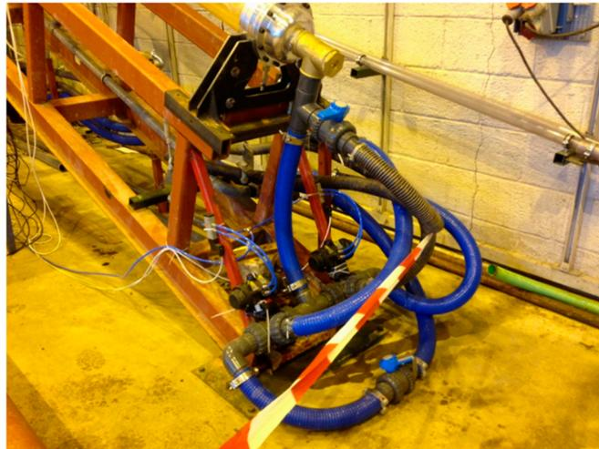
**Figure 5.** Piping and valves at inlet to test section. The valves V1 and V2 of Figure 2 were controlled from the PC using pneumatic actuators. A drain valve (blue handle) with corresponding hose (not shown in Figure 2) was used to drain the test section after an experiment.
