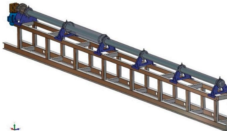
**Figure 1.** Test section with inlet to the right and outlet to the left. A torque motor for the rotating inner pipe is mounted at the outlet.
