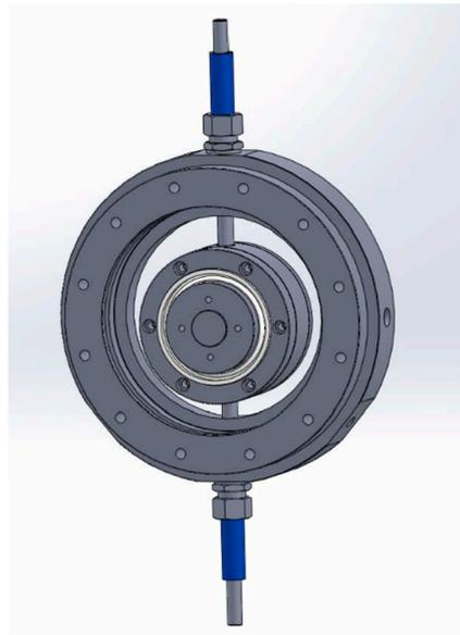
**Figure 4.** Bearing joint connecting two sections of inner pipe.
