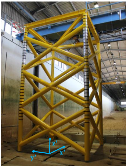
Fig. 2 Instrumented truss structure in the Large Wave Flume FZK and the local coordinate system. Figure used with permission from the WaveSlam project group.
