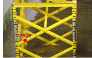
Fig. 13 The location of the bracing force transducer FTBF01 on the truss structure. The hammer test was performed on the same location.
