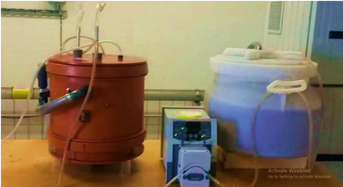
Figure 3.3 Photo of the UASB pilot plant
