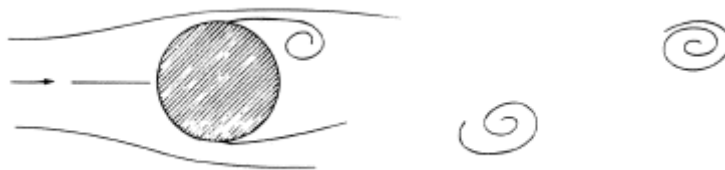
Figure 2.1: Vortex formation behind a circular cylinder (Sunden 2011).
