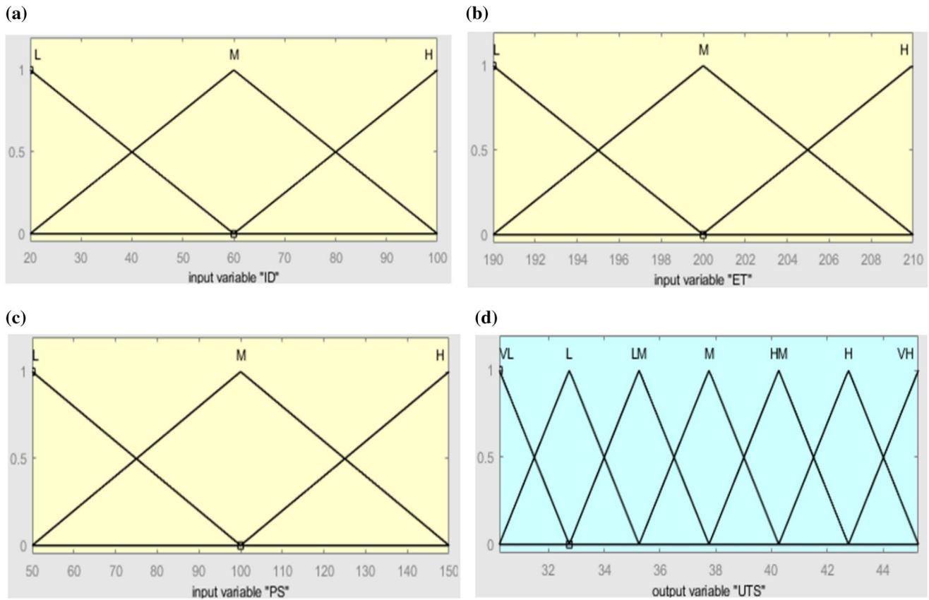
Fig. 3 Triangular MFs of **a** Infill density **b** Extruder temperature **c** Print speed and **d** Tensile strength
