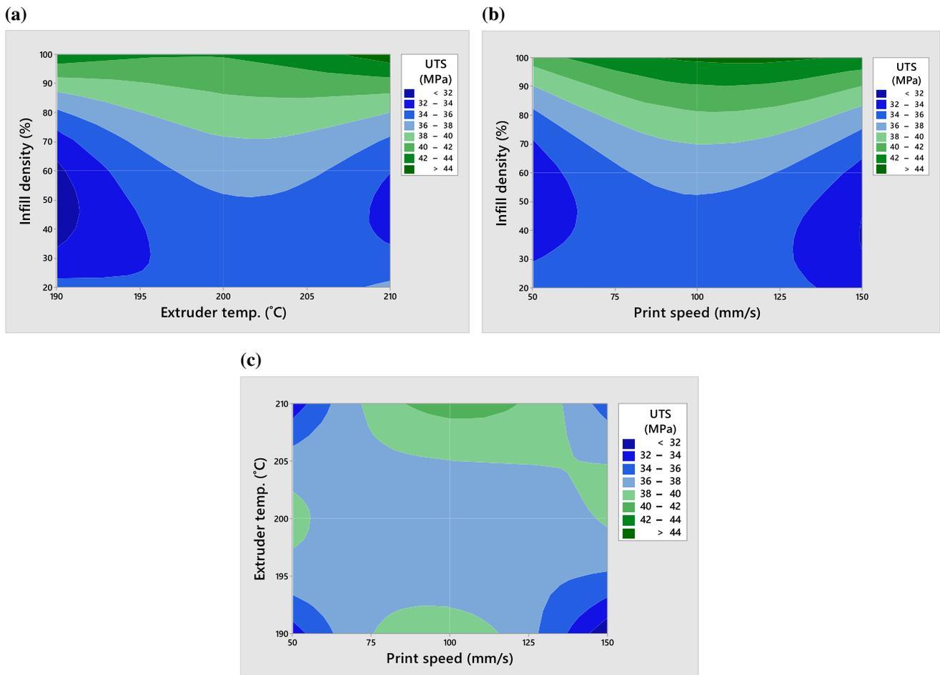
**Fig. 5** Contour plots of **a** infill density (ID) and extruder temperature (ET), **b** infill density and printing speed (PS) and **c** extruder temperature and printing speed with ultimate tensile strength
