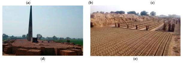
**Figure 4.** Burnt fired clay manufacturing: (**a**) Wet mixing and voids filling of clay. (**b**) Clay lump. (**c**) Sun drying of demolding specimens. (**d**) Fired in standard Hoffmann kiln. (**e**) Mass production of clay bricks.
