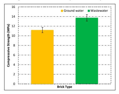
Figure 8. Compressive strength of fired clay bricks.
