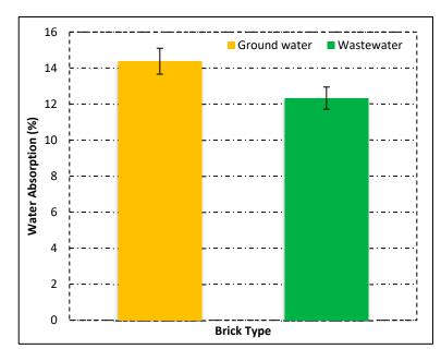
Figure 7. Water absorption of fired clay bricks.
