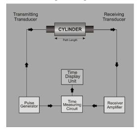
Figure 6. Ultrasonic pulse velocity working flow diagram [43].
