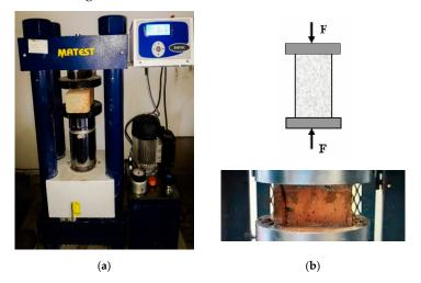
Figure 5. (a) Compression machine with brick. (b) Compressive strength concept.
