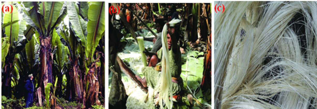
Fig. 1. Extraction of false banana from enset plant manually a). Enset plant b). Manual extraction on plane wood c). Extracted false banana fibre.
