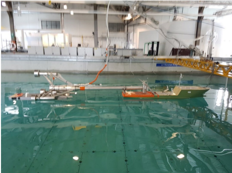
Figure 4. Arrangement of test facilities for the testing of the MINT transport and installation method for wind turbines.
