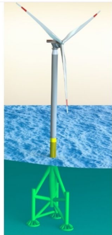
Figure 2. MC-7 Wind turbine for 50 to 120 m water depth.
