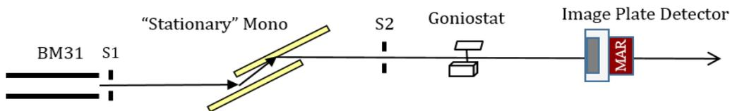
FIGURE 2. These are two experimental setups at BM31, SNBL. (a) depicts schematically the energy scan, (b) is the fixed wavelength  $\omega$ -scan setup which is used for orientational measurements.
