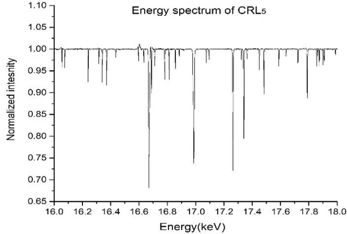
**FIGURE 4.** The transmission spectrum of CRL<sub>5</sub> from the energy scan.
