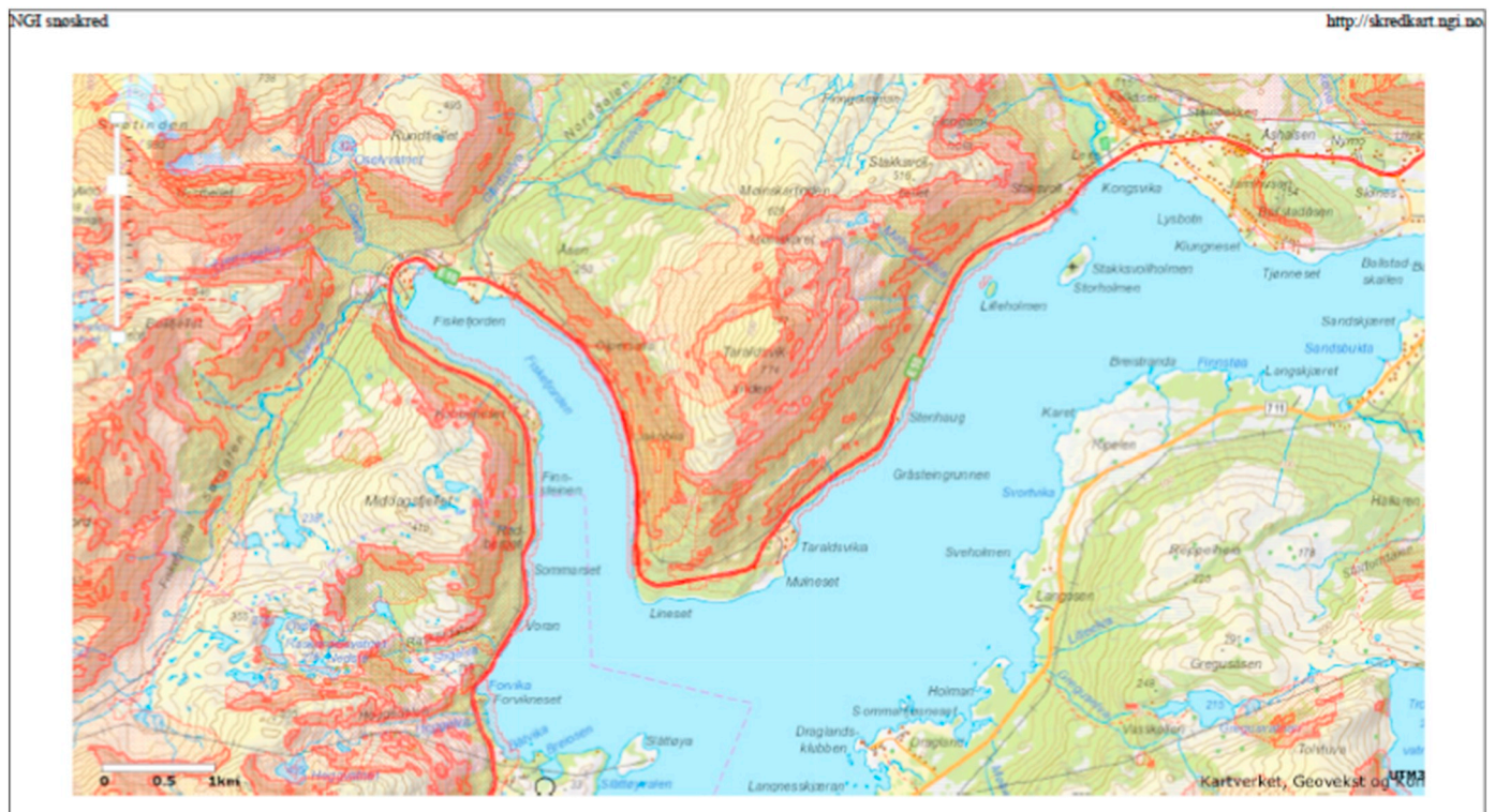
Fig. 3. Example of open source avalanche map of Lødingen, Nordland, North-Norway, provided by NGI. The dark red delineated area represents avalanche release areas (inclinations steeper than 30°). The pink delineated area represents theoretical maximum runout zones. (For interpretation of the references to colour in this figure legend, the reader is referred to the web version of this article.)
