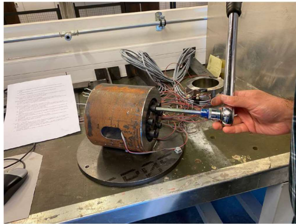
Figure 3.10. Test jig for measuring maximum preload
