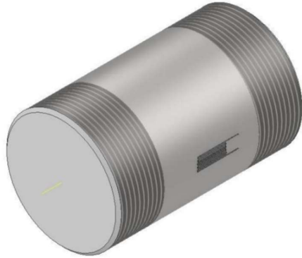
Figure 3.11. Central pin with two strain gauges at 180° distance
