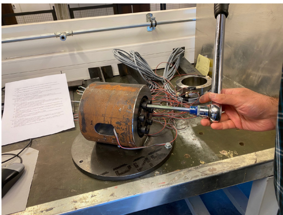
Fig. 4. Experiment setup and manual application of torque on axial-radial pin system in the test jig
