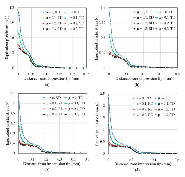
**Figure 12.** Effect of the material anisotropy on the distribution of the equivalent plastic strain along the rolling direction (RD) and transverse to the rolling direction (TR) of the sheet metal at indentation depths of (**a**) 0.025 mm, (**b**) 0.05 mm, (**c**) 0.075 mm and (**d**) 0.1 mm.
