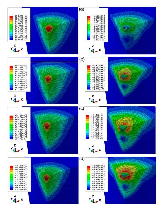
**Figure 14.** Distribution of equivalent stress (in MPa) under maximum displacement (left-hand side) and after unloading (right-hand side) state for the indentation depth of 0.05 mm and friction coefficients: (**a**) 0, (**b**) 0.1, (**c**) 0.2 and (**d**) 0.3.
