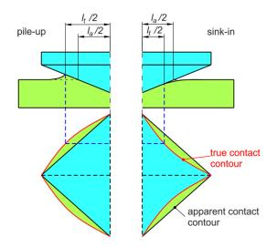
**Figure 1.** Change of the contact contour of the indent due to pile-up and sink-in:  $l_a$ —apparent contact length (mm),  $l_t$ —true contact length (mm).
