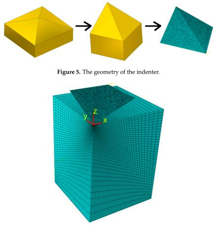
Figure 6. Finite element mesh used in the numerical simulation.
