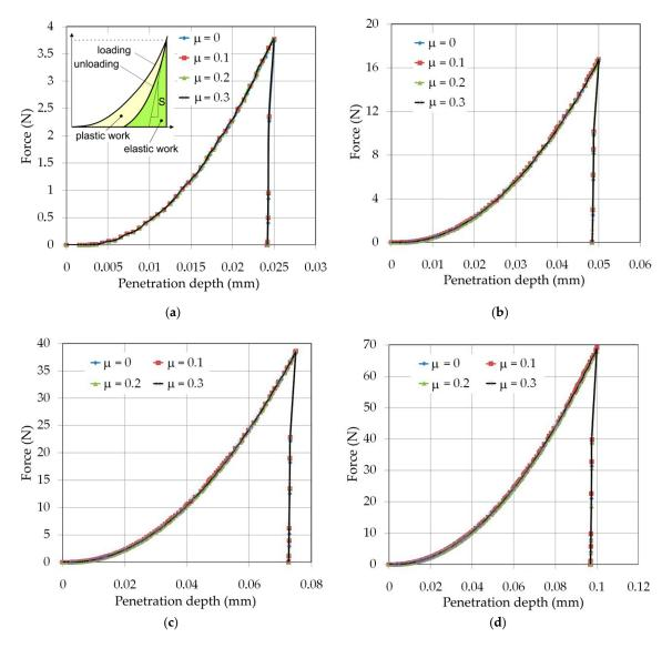
**Figure 11.** Load–displacement characteristics for penetration depths: (**a**) 0.025 mm, (**b**) 0.05 mm, (**c**) 0.075 mm and (**d**) 0.1 mm.
