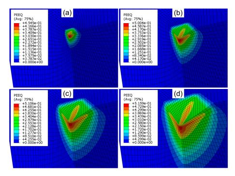
**Figure 8.** Distribution of equivalent plastic strain in the impression area at frictionless conditions and for indentation depths: (**a**) 0.025 mm, (**b**) 0.05 mm, (**c**) 0.075 mm and (**d**) 0.1 mm (identical scales).
