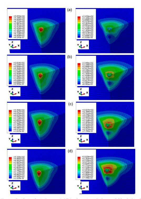
**Figure 13.** Distribution of equivalent stress (in MPa) under maximum displacement (left-hand side) and after unloading (right-hand side) state for the indentation depth of 0.025 mm and friction coefficients: (**a**) 0, (**b**) 0.1, (**c**) 0.2 and (**d**) 0.3.
