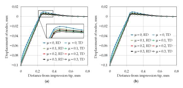
**Figure 10.** (**a**) Displacement of the nodes along RD and TD for indentation depth 0.1 mm, and (**b**) effect of the material anisotropy on the pile-up effect.
