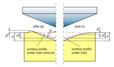
Figure 2. Cross section of the indentation profile, dimensions in (mm).
