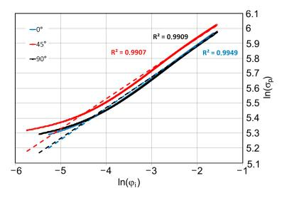
Figure 4. Exemplary strain hardening curves for the specimens cut at 0°, 45° and 90°.
