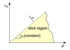
Figure 7. Coulomb friction model representation.
