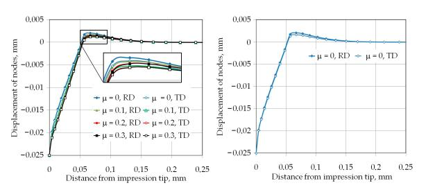
**Figure 9.** (**a**) Displacement of the nodes along the rolling direction (RD) and (TD) for indentation depth 0.025 mm and (**b**) effect of the material anisotropy on the pile-up effect.
