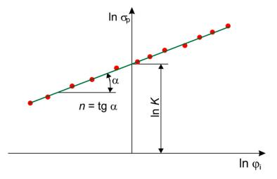
Figure 3. Graphical method of determination of strain hardening parameters.
