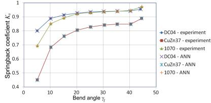
Figure 4. Effect of bending angle on springback coefficient.
