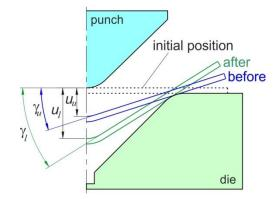
Figure 3. The schematic of measurement of springback.
