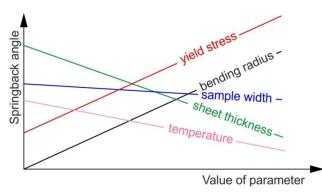
Figure 1. Effect of selected parameters on the springback angle.
