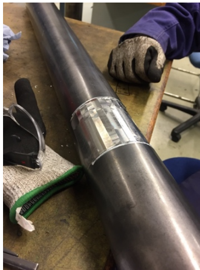
Figure 7. Example of tubular column with simulated corrosion damage by grinding.
