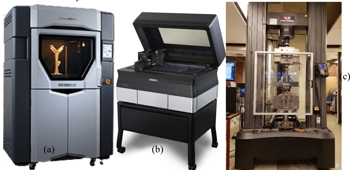
Figure 1. Machines used for additive manufacturing machine and testing (a) Fortus 450mc FDM machine (b) Objet 30 Prime Polyjet machine and (c) Instron 5985 tensile test machine.
