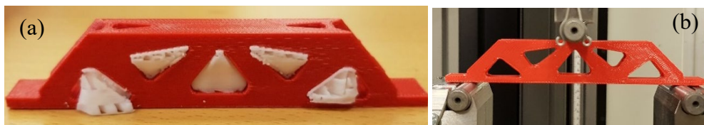
Figure 4. Optimized part (a) as manufactured with material support material and (b) under three-point bending test.
