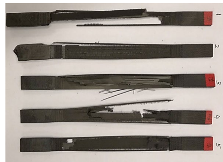
Figure 6. Failed UD tensile samples.
