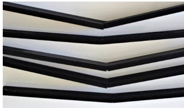
Figure 8. Failed three-point flexural sample.
