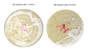
**Figure 3.** Pictures showing salt precipitation on the core inlet when supercritical CO<sub>2</sub> injection rate was increased from (**A**) 1 mL/min to (**B**) 5 mL/min. Increase in CO<sub>2</sub> injection rate decreased the amount of deposited salt.
