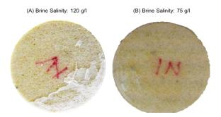
**Figure 4.** Pictures showing salt cake development at the core inlet when brine salinity was decreased from (A) 120 g/L to (B) 75 g/L. Decrease in brine salinity further decreased the amount of deposited salts.
