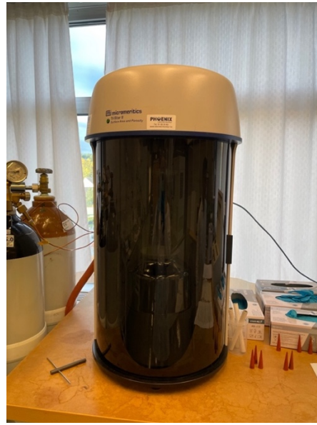
Figure 4.3.5.3. Micromeritics Tristar 2. Surface Area and Porosity
