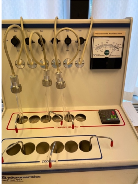
Figure 4.3.5.2 Micromeritics, VacPrep 061. Sample Degas System
