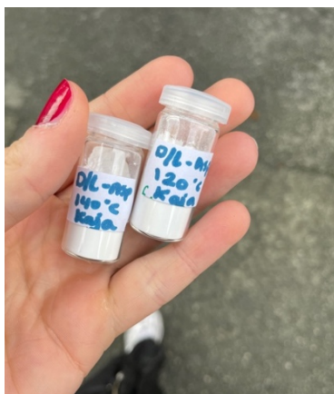
Figure 4.2.2. Autoclaves samples, using DL-Asp and 120°C/140°C.
