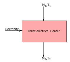
Figure 3. Mass and energy flows through the pellet heating unit.
