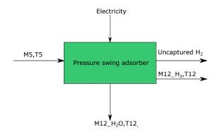
Figure 7. Mass and energy flow through the waste gas separation unit.
