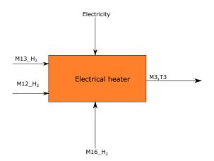
Figure 8. Mass and energy balance through the electrical heating unit for hydrogen stream.
