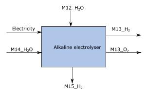
Figure 6. Mass and energy flow through the electrolyzer.
