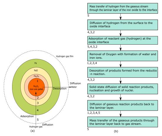
**Figure 1.** (a) Shrinking core model depicting the evolution of iron ore reduction reaction with hydrogen [56]. (b) Process steps in the reduction of iron ore pellets with hydrogen [37]. The location of the process steps is represented from numbers 1 to 5 (1b), which are also depicted in the shrinking core model (1a).
