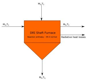
Figure 4. Mass and energy flow through the DRI shaft furnace.
