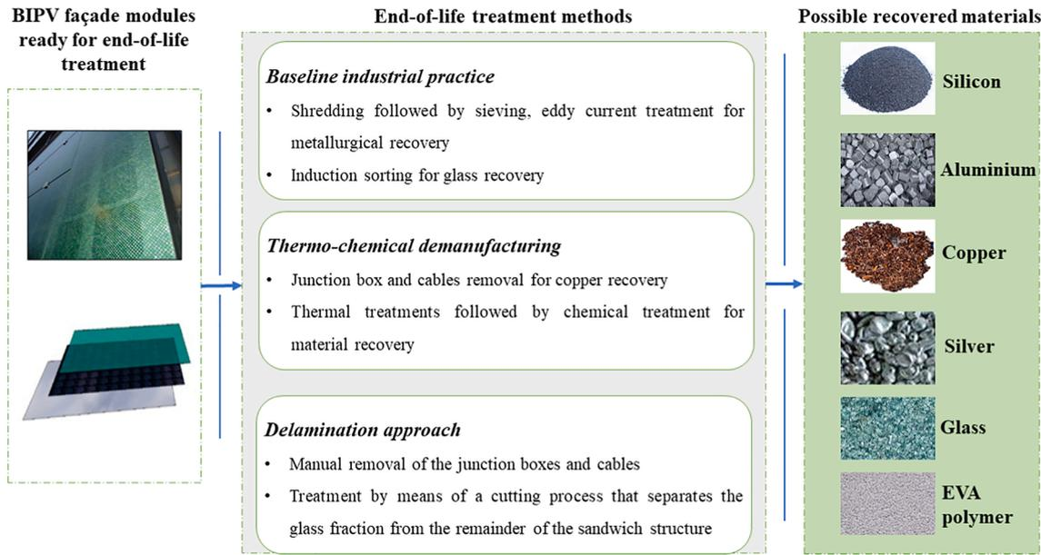
Fig. 3. End-of-life material recovery process for BIPV module.
