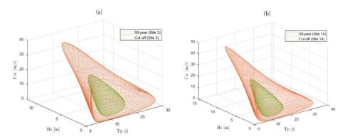
Fig. 6. Environmental contours associated with the ECM 50-years return period and with the wind turbine cut-off wind speed. a) Site 3. b) Site 14 [7].
