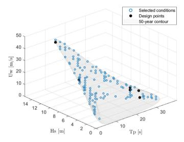
**Fig. 9.** Discretized conditions for 50-years contour surface for site 14. The blue circles are the selected conditions, while the filled black circles are the design points.
