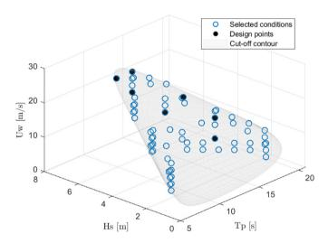
**Fig. 10.** Discretized conditions for cut-off contour surface for site 3. The blue circles are the selected conditions, while the filled black circles are the design points.
