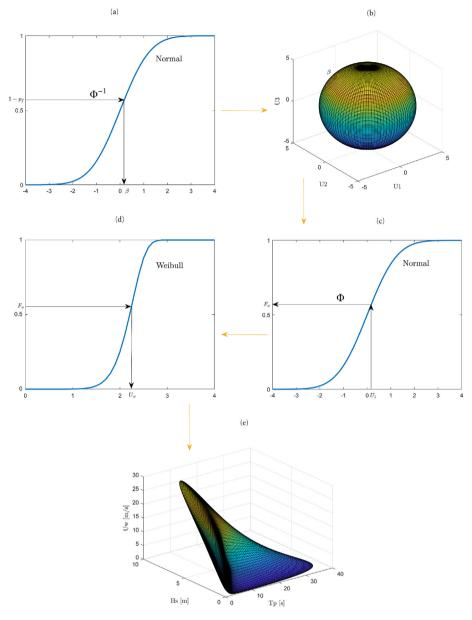
**Fig. 1.** Graphical representation of the Environmental Contour Method (ECM), based on Rosemblatt transformation [12]. Only the marginal (Weibull) distribution of  $U_w$  is shown, relative to a standard height of 10 m and site 14 (Table 3) [7].
