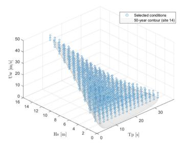
**Fig. 5.** Environmental conditions used for FLTA. The 50-year contour surface of site 14 is included to visualize the threshold of the selected conditions.
