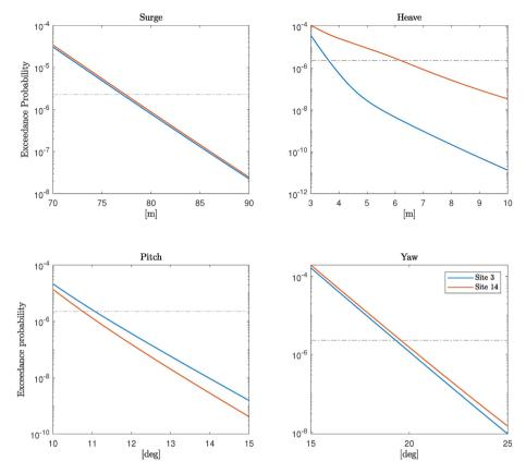
Fig. 7. Full long-term extreme exceedance probability of platform surge, heave, pitch, and yaw motions computed for site 3 and site 14. The dashed line represents the exceedance probability associated with 50-years return period.
