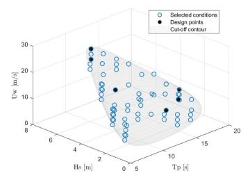
**Fig. 11.** Discretized conditions for cut-off contour surface for site 14. The bluue circles are the selected conditions, while the filled black circles are the design points.
