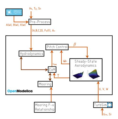
Fig. 3. Flowchart describing the simulation tool structure used in the analysis.
