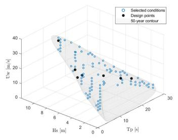
**Fig. 8.** Discretized conditions for 50-years contour surface for site 3. The blue circles are the selected conditions, while the filled black circles are the design points.
