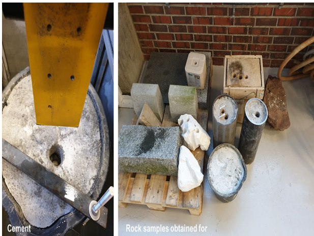
Fig. 3 Collection of different rock specimen drilled to gather experimental drilling data
