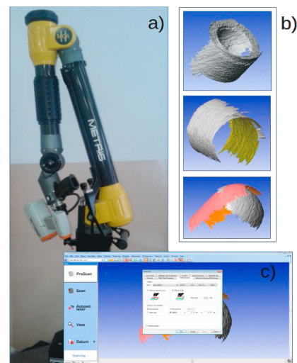
Fig. 11. Application of measuring arm: a) measuring arm, b) digitized grinding pins, c) software settings.
