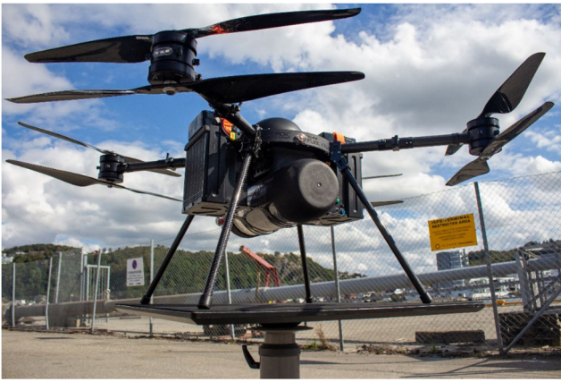
Fig. 2 Staaker BG-200 FC from Nordic Unmanned with the reference fuel cell hybrid system installed
