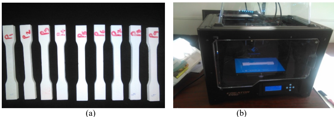
Figure 2. (a) Parts fabricated by FDM machine; (b) FDM Flash forge creator pro
