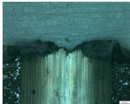
Figure 11 Bur after machining
