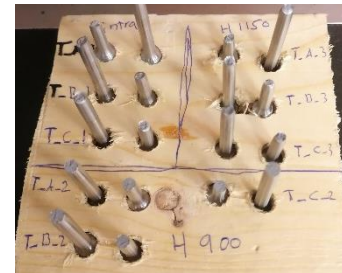
Figure 16 Broken tensile samples
