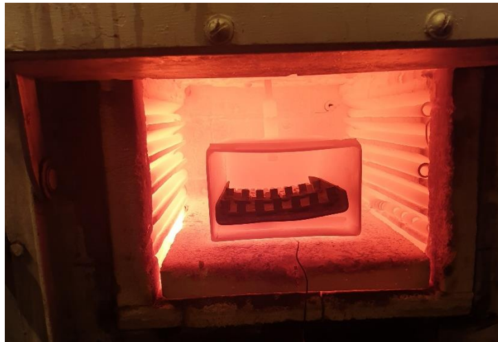
Figure 9 Removing the samples from the oven after solution treatment.
