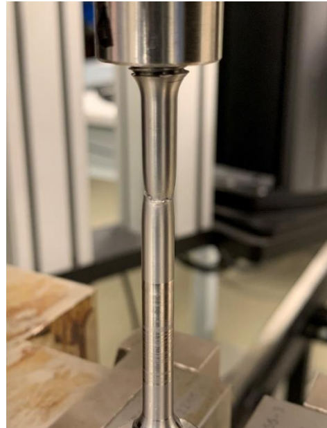
Figure 15 Tensile test post fracture
