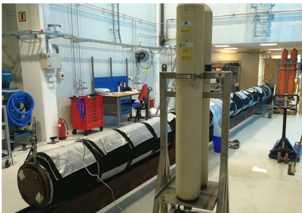
Fig. 4 Positioning of Fish 11 for permeability characterization using the pressure-pulse decay method. The two bottles at either end of the joint correspond to upstream and downstream reservoirs required for the transient pressure testing.
