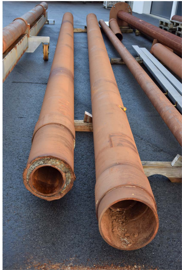
Fig. 1 Two cut and pulled sections from a North Sea well. The Fish 11 is shown to the left.
