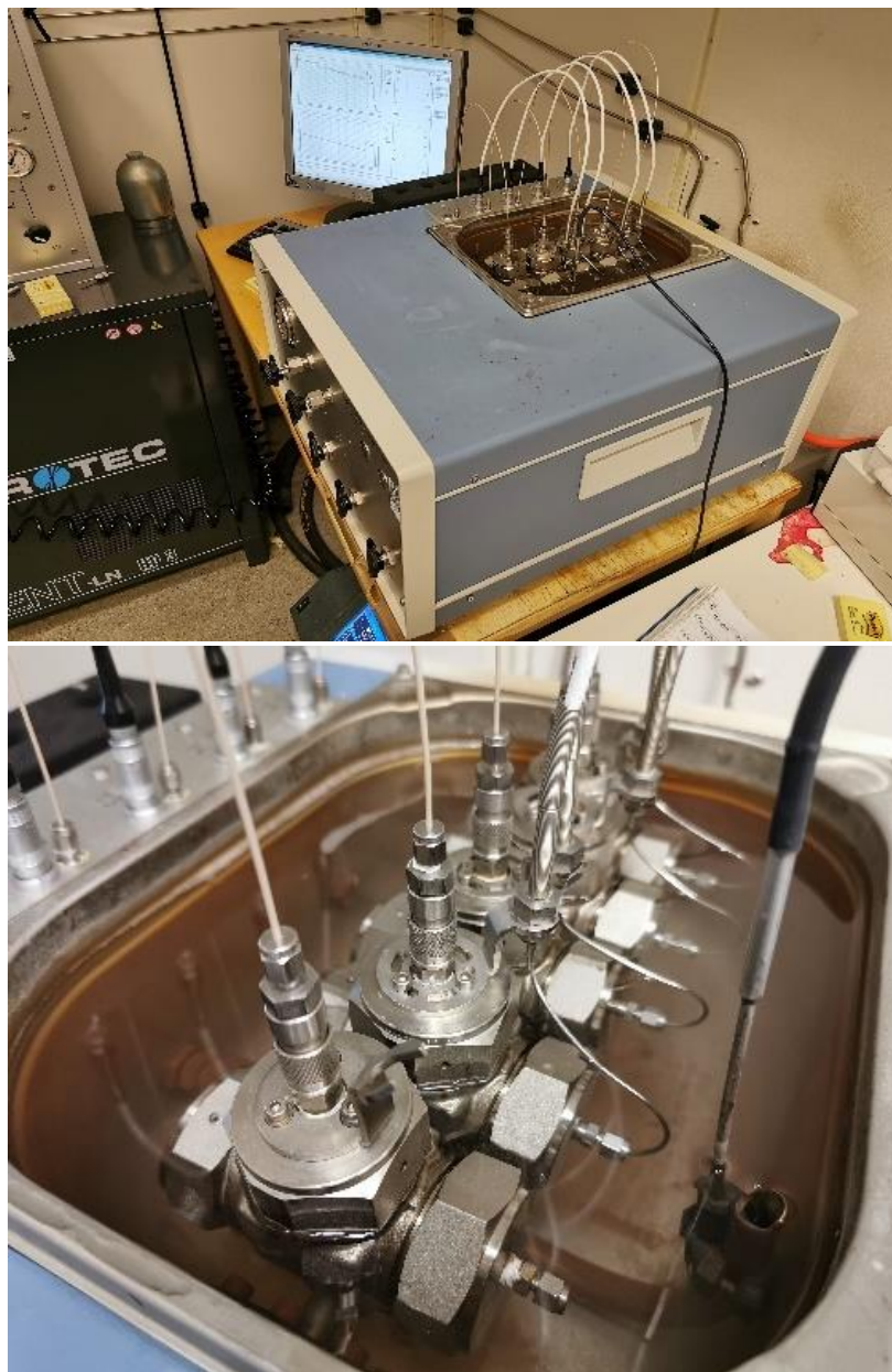
Figure 2.3. Top: The RC5 apparatus in its operational status. Bottom: Closeup of the five cells positioned in the water bath of the RC5 apparatus.
