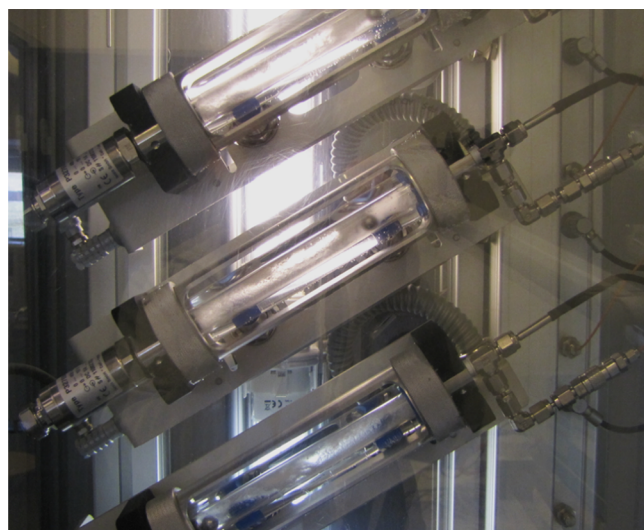
Figure 5. RCS20 rocker rig showing hydrate formation in three of the six sapphire cells.
