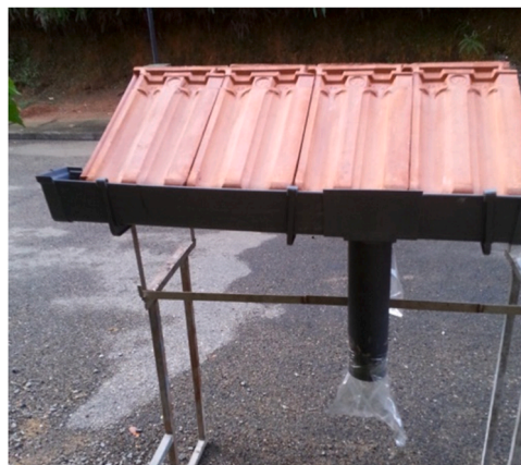
Fig. 3. Roof structure to collect runoff water.
