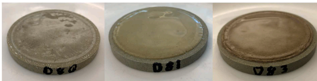
Fig. 9. From left: Residue from Fluid 1 (Disc 2) after total loss, and filter-cakes from Fluid 2 (Disc 4) and Fluid 4 (Disc 8).
