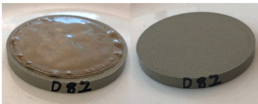
Fig. 10. Disc 7, from testing of Fluid 3 with filter-cake (left) and after filter-cake had been lifted by reverse flow (right).
