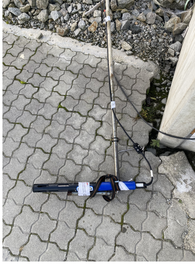
Figure 3.4: YSI sonde secured to steel bar.
