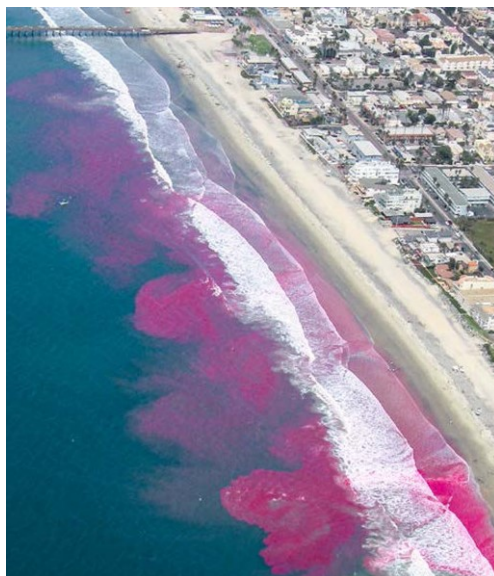
Figure 2.11: RWT released at Imperial Beach, California. Clark et al. (2014) used RWT to study dispersion and transport in the surfzone near shore.
