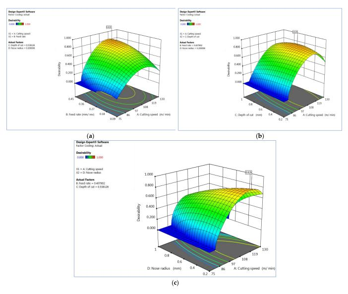
**Figure 5.** Estimated surface plots on desirability (**a**)  $V_c$  vs.  $F_z$ , (**b**)  $V_c$  vs.  $D_c$  and (**c**)  $V_c$  vs.  $R_n$ . Plots produced using Design-Expert software V11 (StatEase, Minneapolis, MN, USA).
