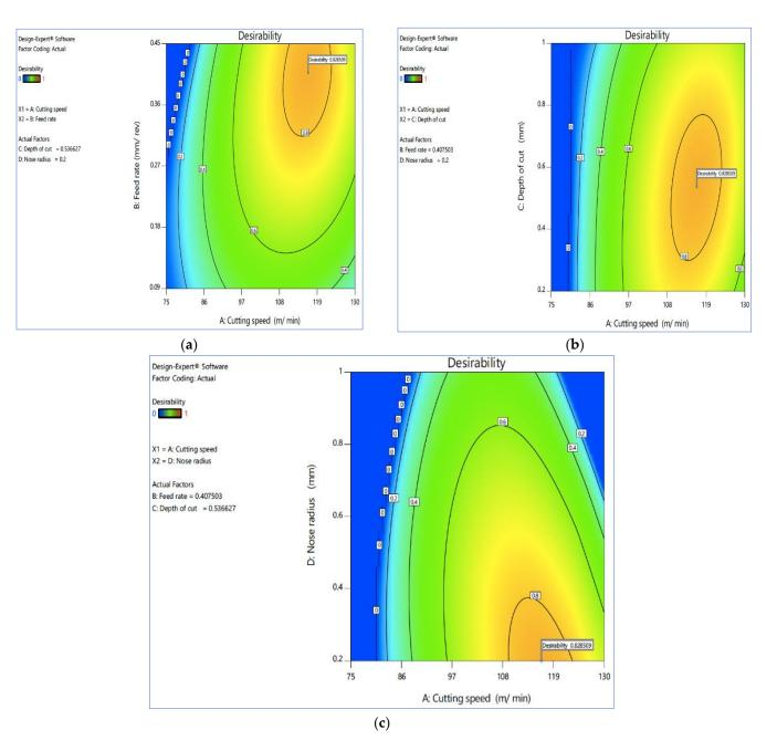
**Figure 6.** Contour plot on desirability for (**a**)  $V_c$  vs.  $F_z$ , (**b**)  $V_c$  vs.  $D_c$  and (**c**)  $V_c$  vs.  $R_n$ . Plots produced using Design-Expert software V11 (StatEase, Minneapolis, MN, USA).
