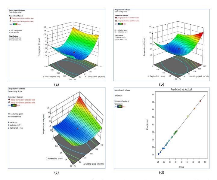
**Figure 3.** Interaction effect of temperature (**a**)  $V_c$  vs.  $F_{z_r}$  (**b**)  $V_c$  vs.  $D_{c_r}$  (**c**)  $V_c$  vs.  $R_n$  and (**d**) actual vs. predicted plot. Plots produced using Design-Expert software V11 (StatEase, Minneapolis, MN, USA).
