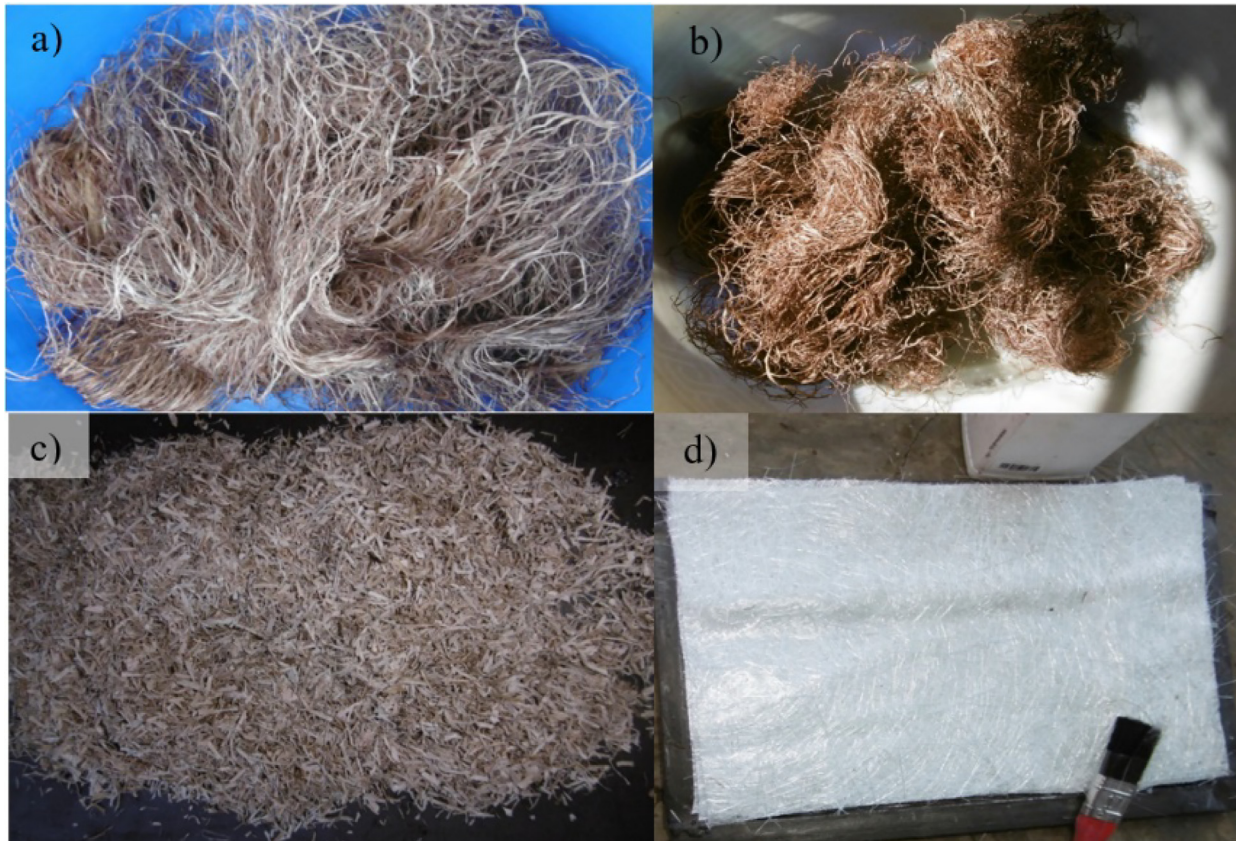
Fig. 1. a) Untreated water hyacinth fiber b) NaOH treated of water hyacinth fiber c) Chopped water hyacinth fiber d) E-glass Fiber.
