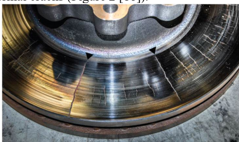
Fig. 2. Radial thermal cracks due to hard braking in heavy vehicle
