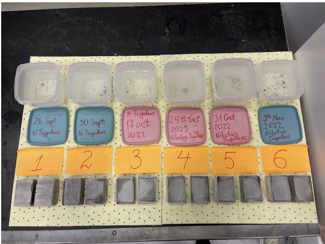
Figure 95: Pairs of concrete sample blocks from rectangular pushout test now used in conventional friction test
