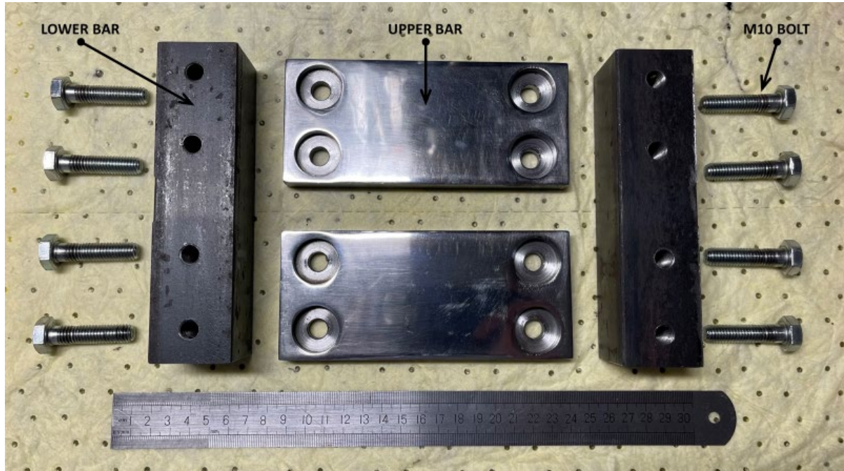
Figure 45: Collection of the parts that are making up the base
