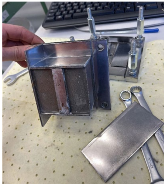
Figure 80: Bottom plate removed from the molding construction and cement sample got exposed
