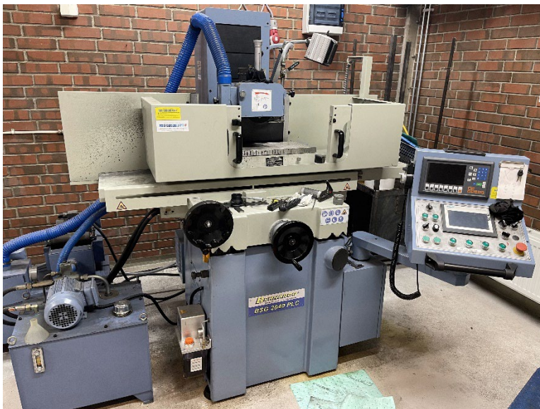
Figure 65: Surface grinding machine Bernardo BSG 2040PLC
