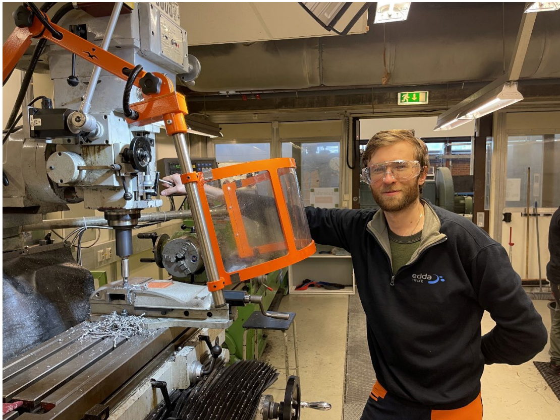
Figure 41: Counterboring process performed by an Author using conventional milling machine
