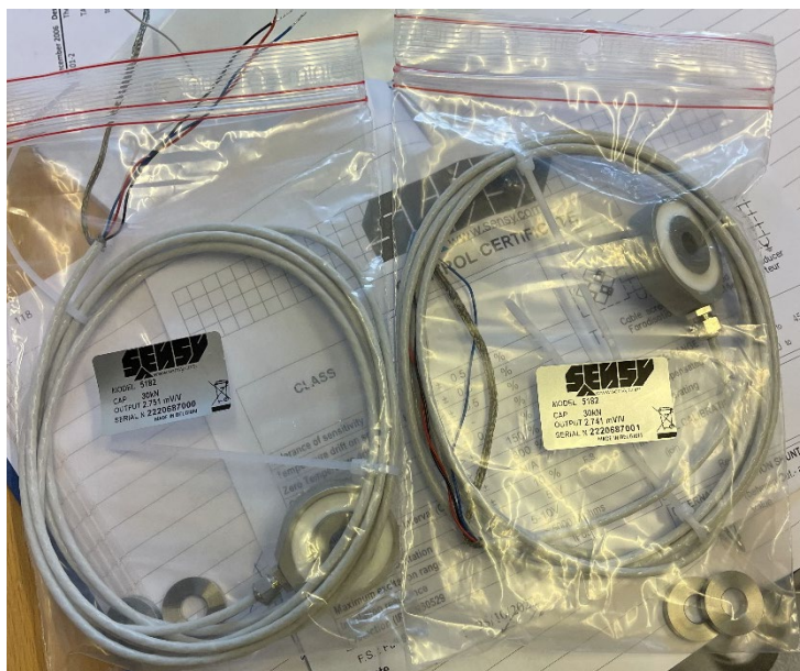
Figure 54: Compression washer load cells in their original package
