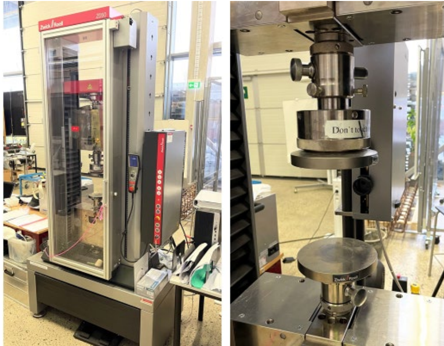
Figure 68: Universal testing machine Zwick/Roell ProLine Z050 with Xforce K load cells
