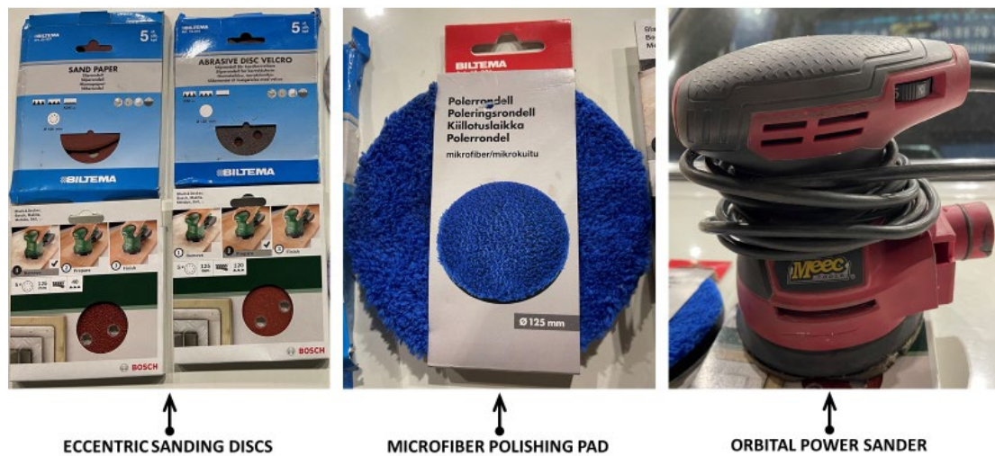
Figure 30: Sanding and polishing equipment
