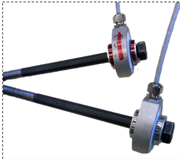
Figure 56: Load cell attached on the bolts including washers
