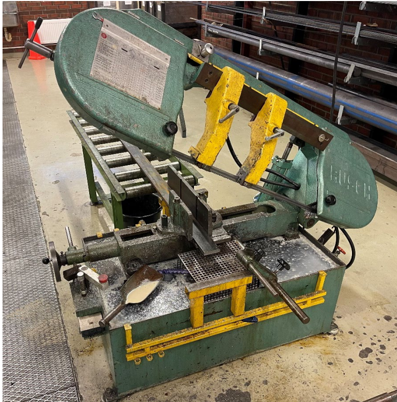
Figure 28: Horizontal metal cutting band saw machine Rusch
