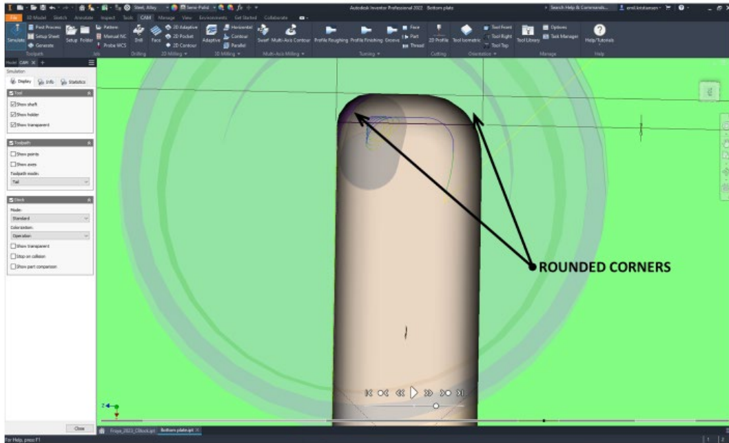
Figure 24: Running toolpath simulation in Autodesk Inventor CAM software revealing hiccup
