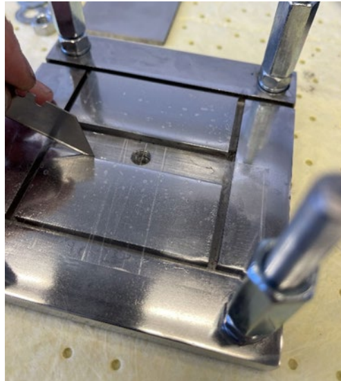
Figure 76: Cutting the excess from the tape applied to surfaces of the bottom plate contacting cement
