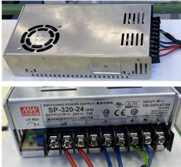
Figure 60: Switching power supply Mean Well model SP-320-24
