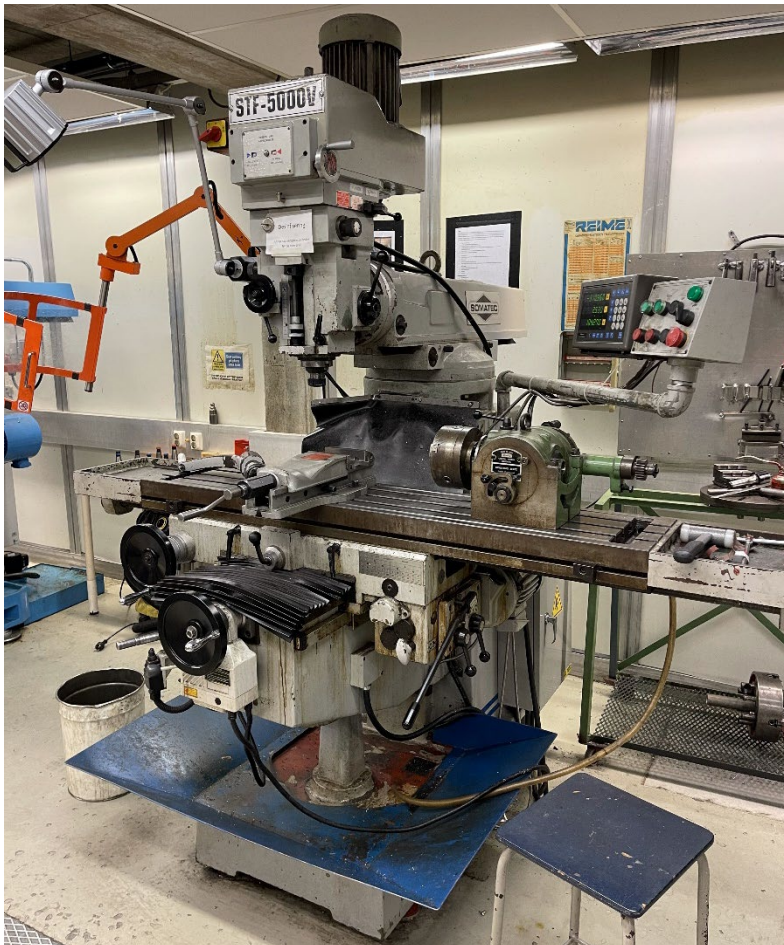
Figure 29: Conventional milling machine Luna STF-5000V
