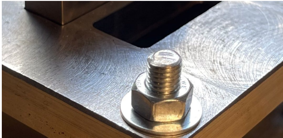
Figure 26: Freshly machined surface of the top plate out of CNC machine
