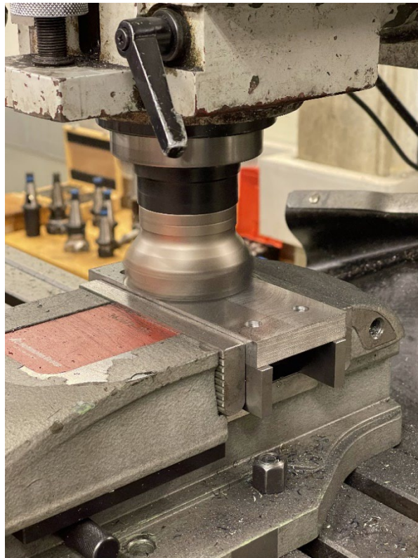
Figure 44: Facing process performed on the largest surface of upper bar
