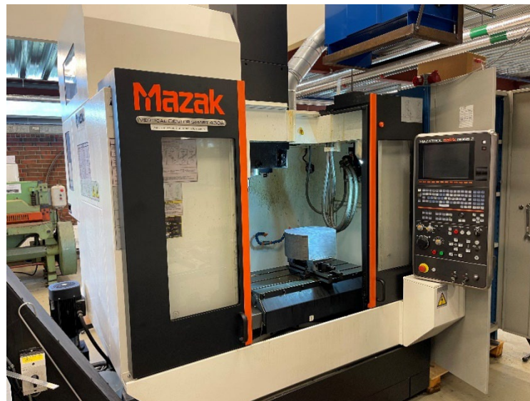
Figure 23: CNC milling machine Mazak
