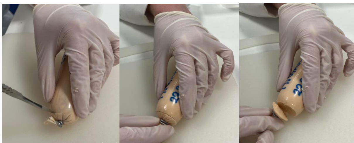
Figure 5. The samples were cut into 1 cm slices using a scalpel prior to the measurements
