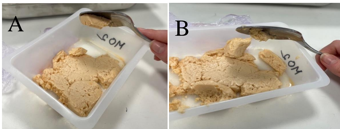
Figure 29. Spoon Tilt Test is done on Farinex product with 1% oil for a product with heat treatment, showing the product covering half of the spoon in A. Picture B shows that most of the product fell off the spoon, with only a tiny amount clinging to the spoon. The temperature measured before the test was 32.7°C.
