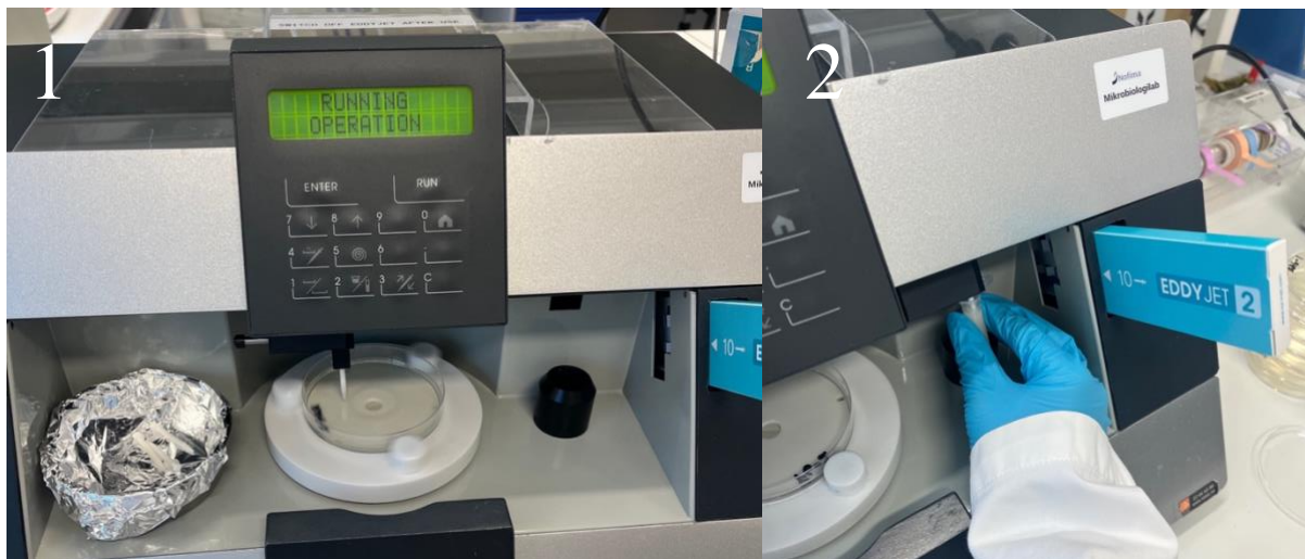
Figure 7. 1 shows the sample spread on a petri dish. 2 shows the automatic plater picking a sample from the sterile tube.
