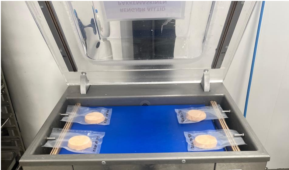
Figure 10. The pucks are single-packed in a plastic bag to be vacuumed before being stored at 4°C for thawing.
