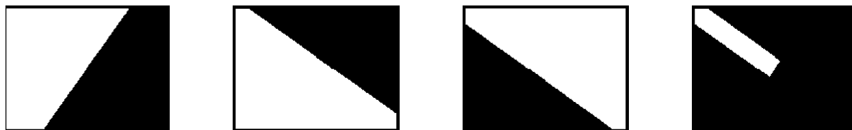
Figure 7.7: Regions created and intersected to create tunnel vision to be applied to images.
