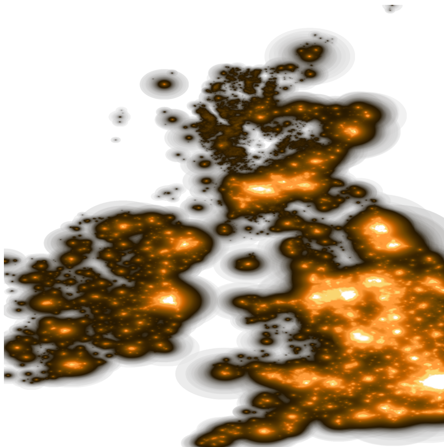
Figure 5.3: Image of United Kingdom light pollution levels using a gradient which emulates light emission, excluding values below 10 (not calibrated)
