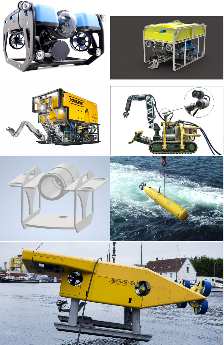
Figure 17: The different ROV classes
