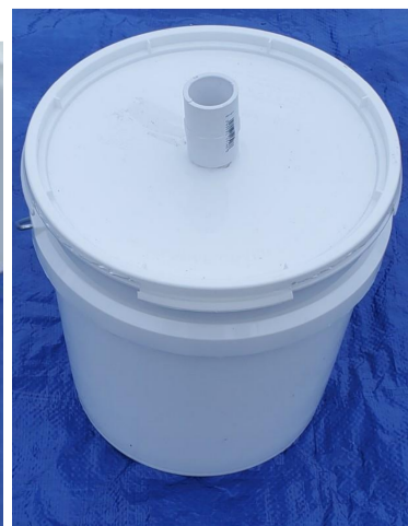
(b) Connection for sample extraction
