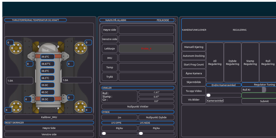
Figure 5.1: Leakage alarm going off in the GUI.
