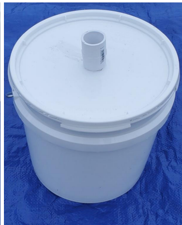
(b) Connection for sample extraction
