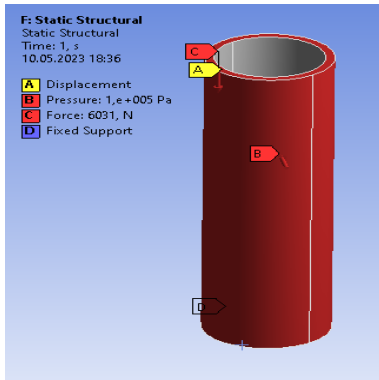
Figure 6.30: Forces and supports on float
