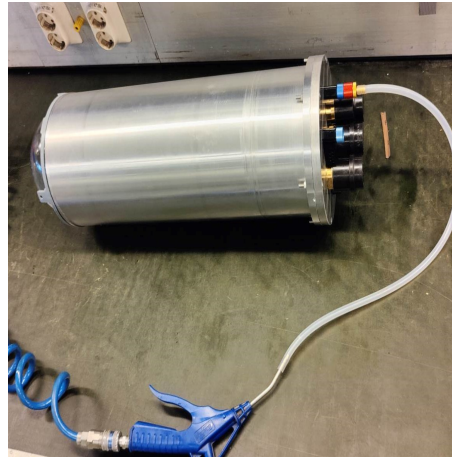
Figure 7.21: Pressure testing of electronic enclosure
