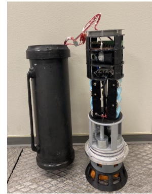
Figure 7.25: Float - Watertest ballast
