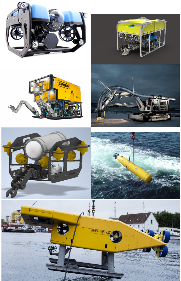
Figure 1.17: The different ROV classes
