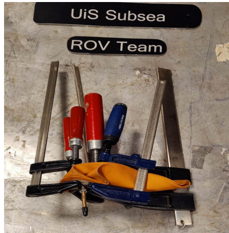
Figure 7.14: Retrofitting of bicycle valve
