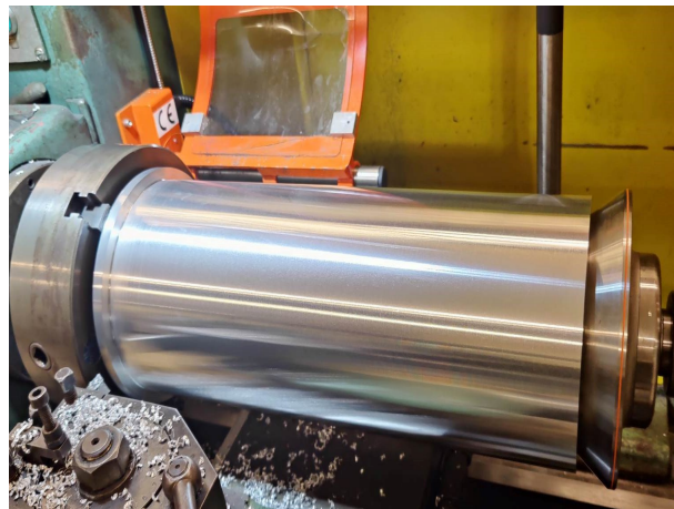
Figure 7.6: Turning off electronic enclosure
