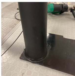
Figure 7.11: Float Top-cap weld
