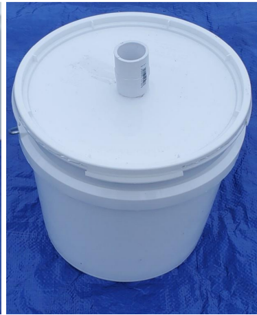
(b) Connection for sample extraction
