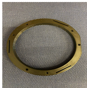
Figure 5.30: End piece of internal electrical components
