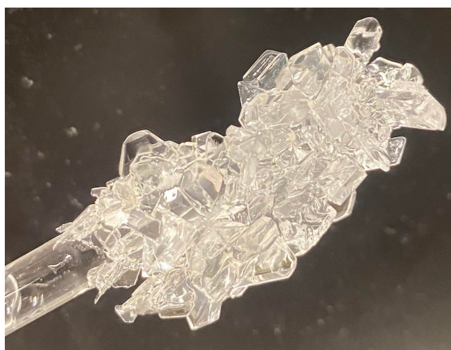
Figure 3.21 THF hydrate crystal growth of N-butylpyrrolidine oxide (4000 ppm).
