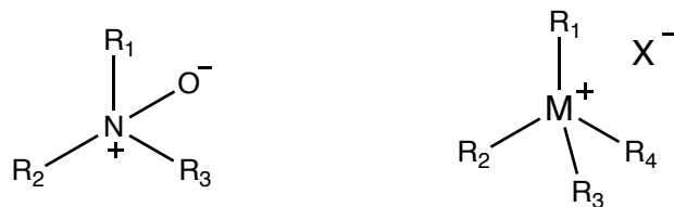
Figure 1.6 General structures of tertiary amine oxide (left) and quaternary -onium surfactant (right), M = N or P, X = counterion, R = alkyl group
