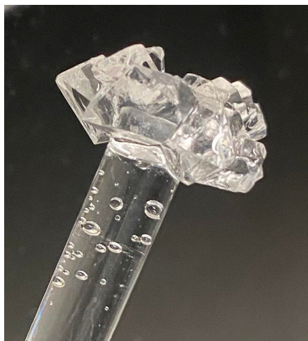
Figure 3.20 THF hydrate crystal growth of Di-iso-pentylcycloheptylamine oxide (1000 ppm)
