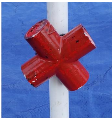
(a) Biological material on structure
