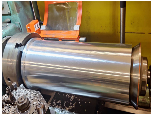
Figure 7.6: Turning off electronic enclosure
