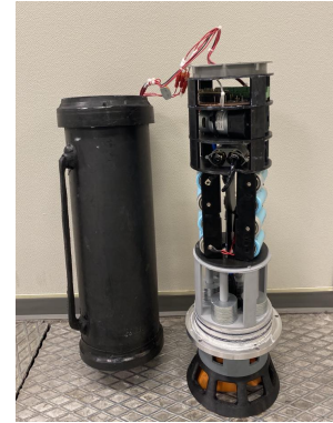
Figure 7.25: Float - Watertest ballast
