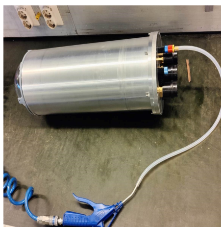
Figure 7.21: Pressure testing of electronic enclosure
