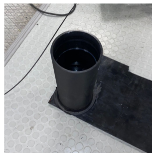
Figure 7.12: Weld water test
