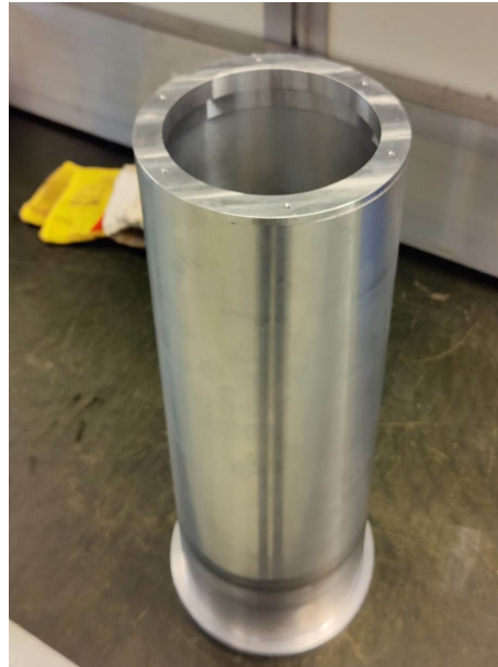
Figure 7.8: Final fit after press fit
