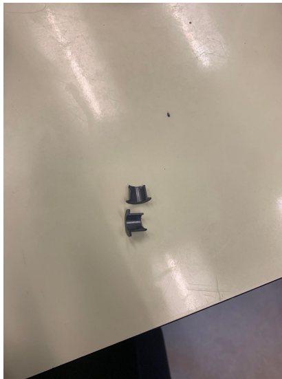
Figure 5.9: Broken plastic bearing
