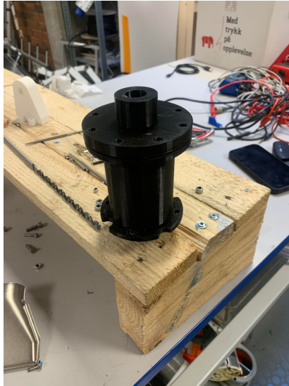
Figure 5.3: 3D printed motor housing
