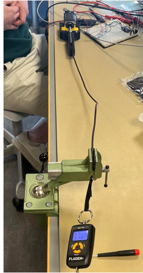
Figure 5.6: Testing of NEMA17 pull force
