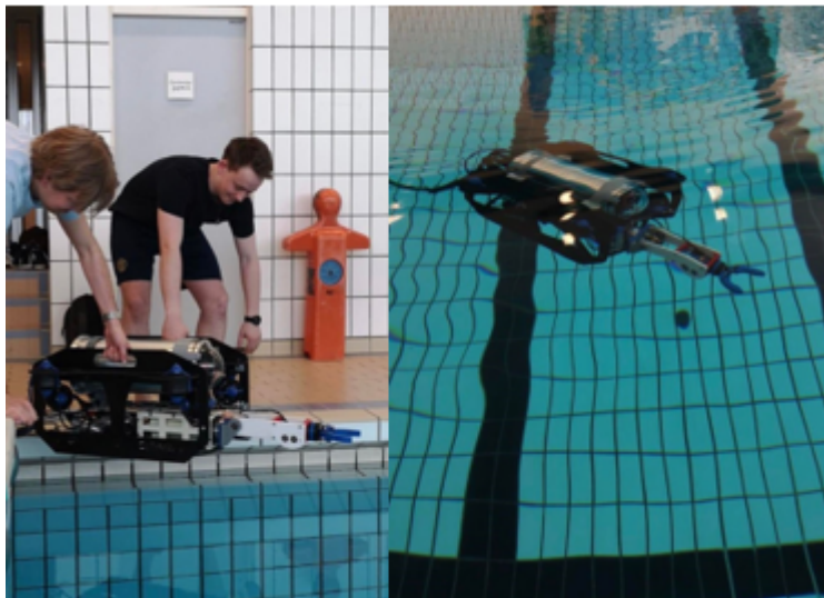
Figure 5.14: Water testing of ROV and manipulator
