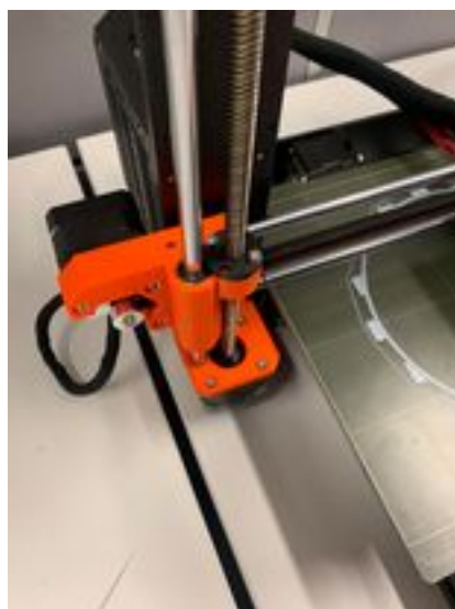
Figure 4.7: 3D-Printer lead screw actuation
