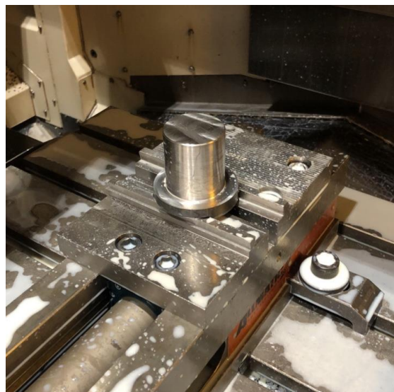
Figure 33, Manufacturing - Welded piston plug
