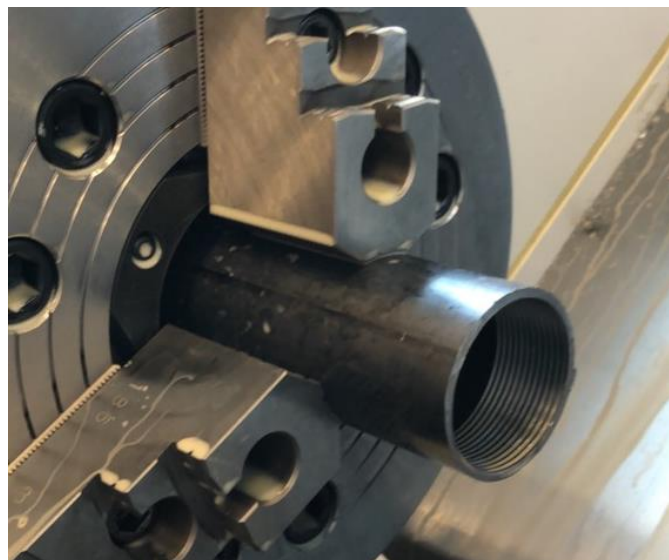
Figure 25, Manufacturing - Outer piston tube
