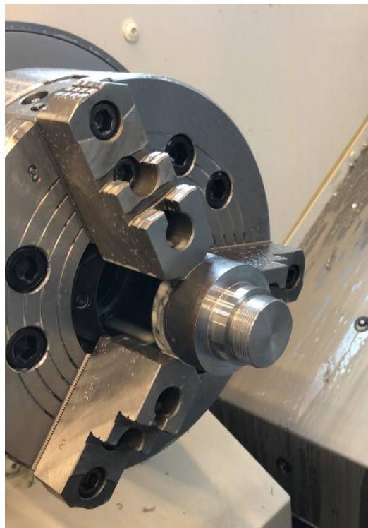
Figure 24, Manufacturing - Piston lock stopper
