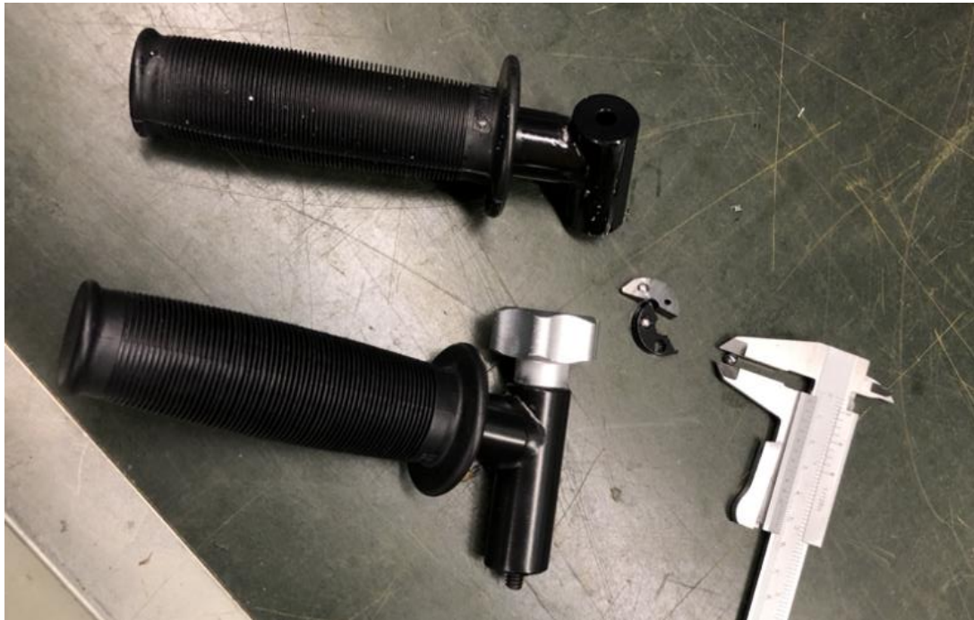
Figure 15, Measuring steel ball from Hytorc handle
