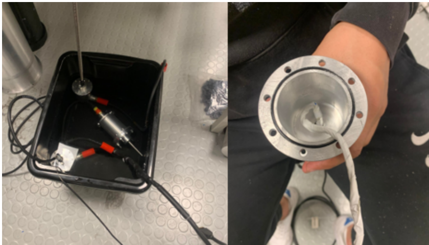
Figure 5.13: Waterproof test of motor housings
