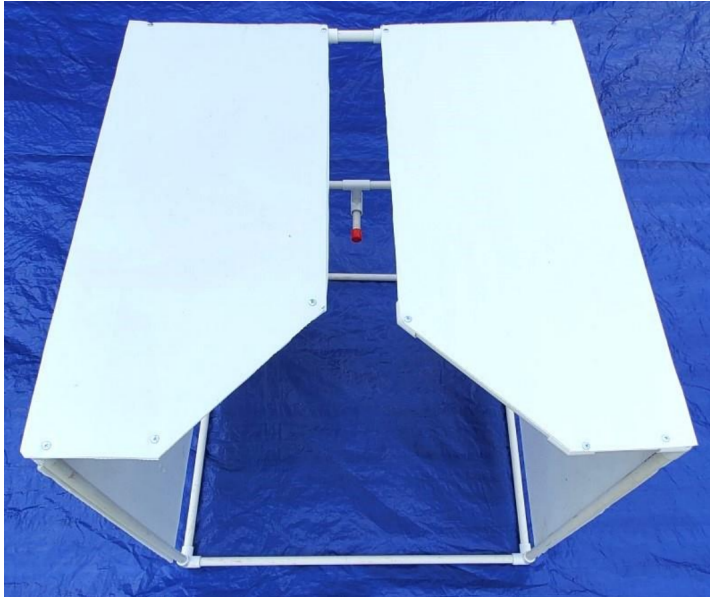
Figure 1.15: ROV Docking station
