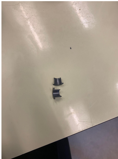
Figure 5.9: Broken plastic bearing
