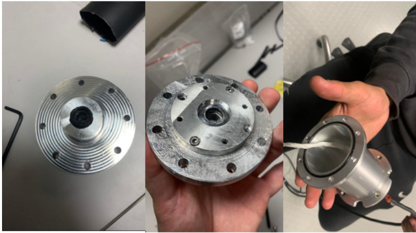
Figure 5.4: Motor housing components with O-ring and shaft seal.
