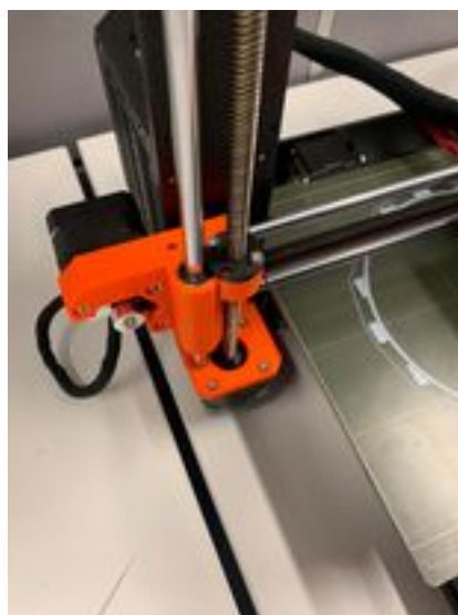
Figure 4.7: 3D-Printer lead screw actuation
