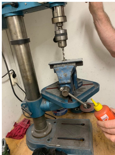
Figure 5.5: Use of pillar drill to increase bore diameters
