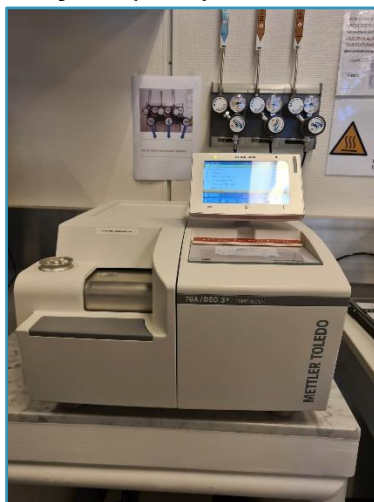
Figure 4-2. TGA instrument used to assess the thermal stability
