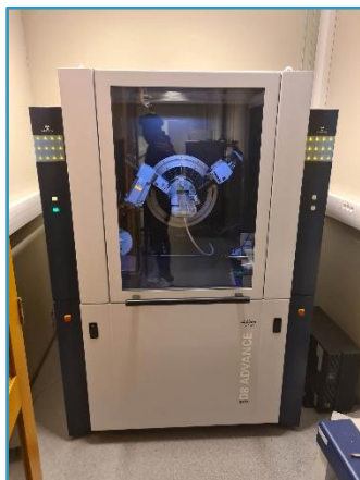
Figure 4-1. XRD instrument to characterize the crystal structure
