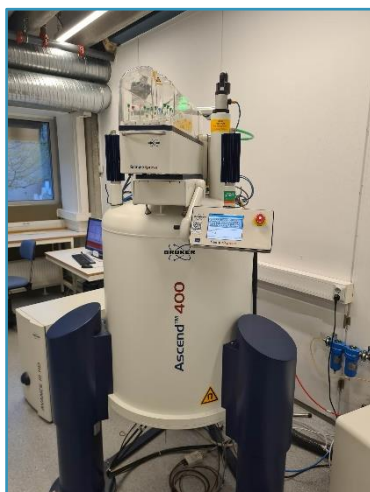
Figure 4-5. NMR instrument used to quantify exchange and loading of ligands and functional groups
